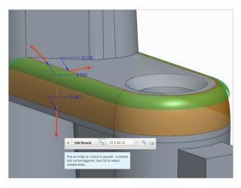
Quickly move geometry using the intuitive 3D dragger with automatic round and chamfer handling.
